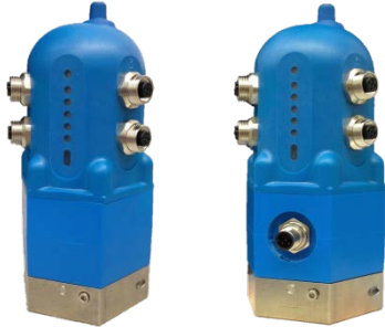
wSIM device with Zone 0 battery module and Zone 0 External Power Module
