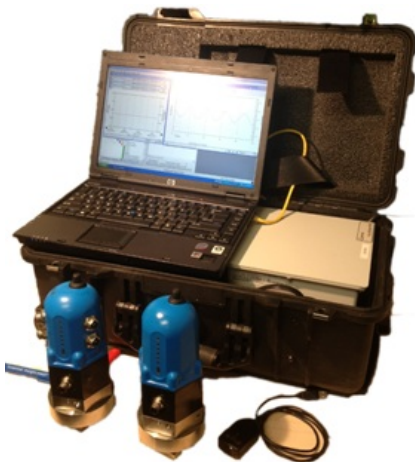
"Prowler" portable wireless data collector kit
