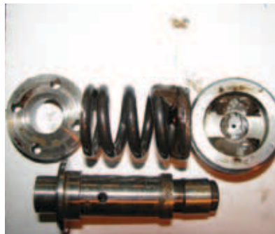
Sludge in trip bolt mechanism.
